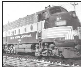
These two first generation units are mechanically identical. The F7A at left was quickly improved to provide better access and visibility with an external walkway: Namely a GP7. Howard Ameling
